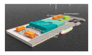
The island's HVAC infrastructure also includes five modules or substations (shown in orange and fluorescent green in the diagram opposite), which will be installed directly on the island structure. These substations will contain equipment such as transformers and gasinsulated switchgear (GIS) substations.
