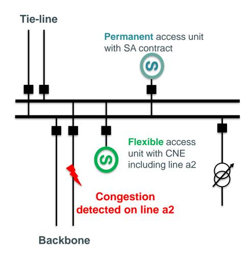
In **real-time**, if the congestion that was not forecasted in DA/ID, is measured on line a2,
