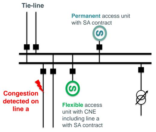
In **DA & ID CRI determination process**, if a congestion is forecasted on line a (monitored by CRI & Gflex), even after application of Elia internal RA,
