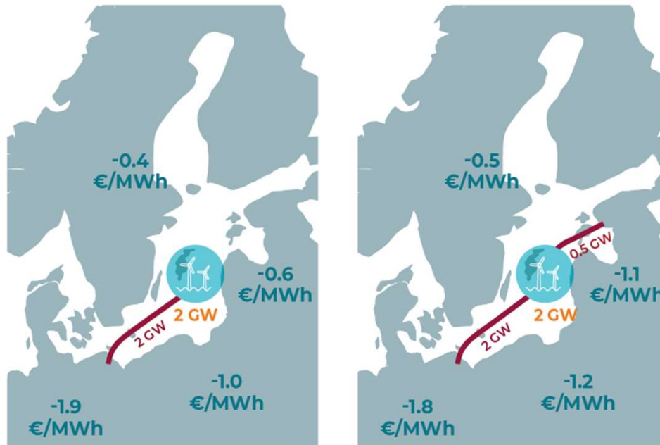
Price effect of an additional 2 GW cross-border radially connected offshore hub in the Baltic Sea in the 2023 day-ahead market
