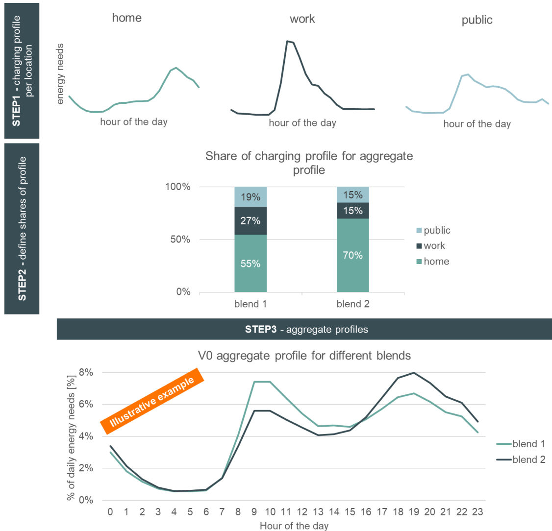
Figure D-2: Illustrative profile for the construction of the V0 aggregate profile, based on individual profiles of home, work & public charging.
