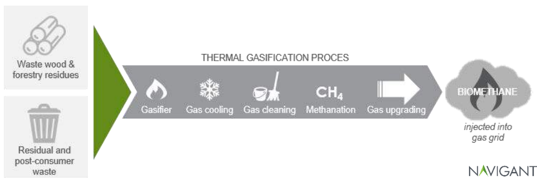
Figure 8 Schematic overview of the thermal gasification process
