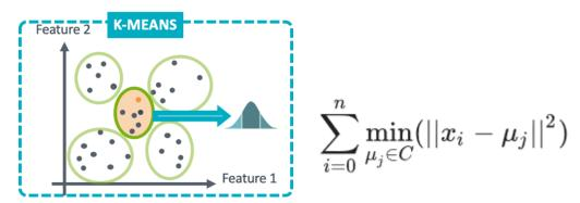
In each cluster, the probabilistic distribution of LFC block imbalances of the periods associated with each cluster is calculated. During the day-ahead calculation of the FRR reserve capacity needs, it is determined for each quarter-hour to which cluster the corresponding day-ahead prediction of features is associated. This determines the relevant LFC block imbalance distribution representing the prediction risk.
