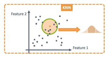
During the day-ahead calculation of the FRR reserve capacity needs, the relevant LFC block imbalance distribution representing the prediction risk is calculated based on the relevant 3500 nearest neighbours.
