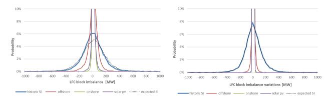
Figure 8 : Extrapolation of the LFC block imbalance towards the expected LFC block imbalance (SI) for 2020
