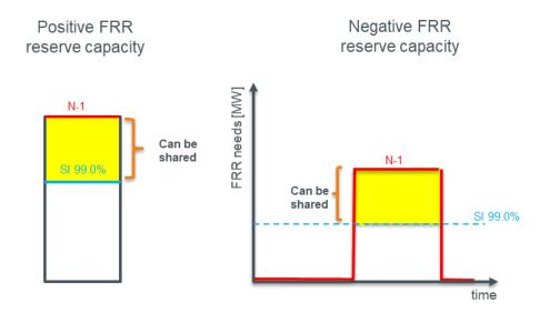
Figure 10 : Visual representation of the maximal sharing potential following SOGL by the surface between dimensioning incident (N-1) and historic LFC-block imbalances (SI 99%) for dimensioning positive FRR needs (left) and negative FRR needs (right)
