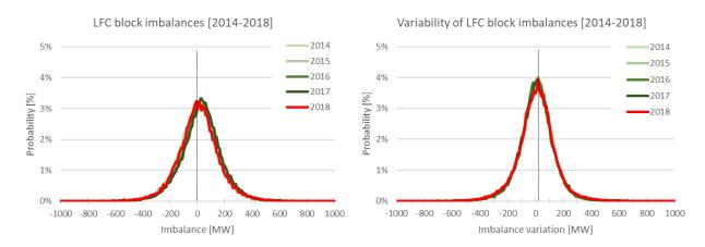
Figure 7 : Probability distribution of the LFC block imbalances between 2014 and 2018 (in steps of 10 MW)
