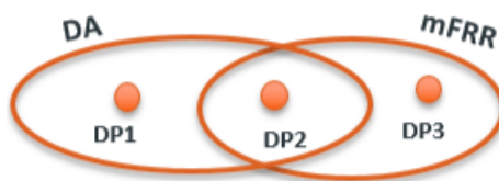
Figure 3 : Overlapping pools for a Combo between DA and mFRR. DP 1 and DP 3 are Pure Delivery Points, DP 2 is a Combo Delivery Point.
