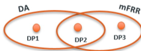
Figure 4 : Overlapping pools for a Combo between DA and mFRR. DP 1 and DP 3 are Pure Delivery Points, DP 2 is a Combo Delivery Point.
