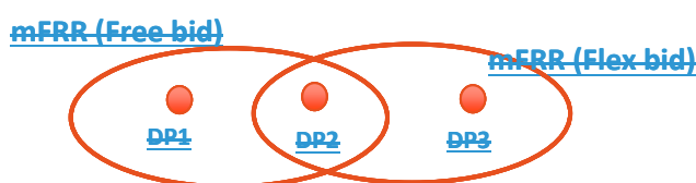
Figure 3 : Overlapping pools for a Combo between non-reserved mFRR and reserved mFRR Flex. DP 1 and DP 3 are Pure Delivery Points, DP 2 is a Combo Delivery Point.
